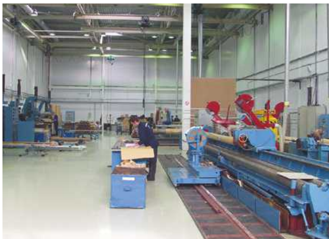
Fig. 8. Shop area of 40.5-800 kV paper insulation winding at the Izolyator plant
