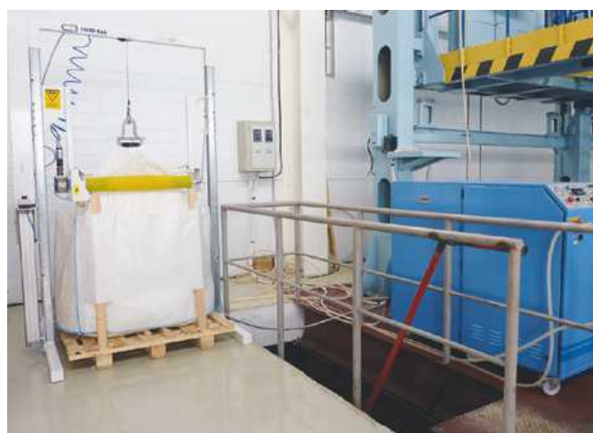
Fig. 12. Unit for degassing and metering feed of compression gel at the Izolyator plant
